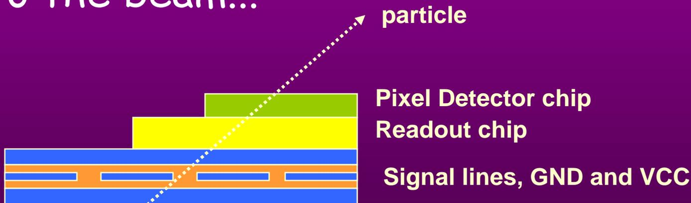
... so it is important that particles are not blocked by the ground and power metal planes.
