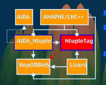
Defines the ntuple as a data type low-level creation, updating and navigation interface Implemented using our tag model
